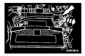
1. Disconnect the secondary positive cable from the primary battery terminal.
