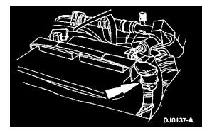
2. Wrap the secondary positive cable with a non-conductive material to insulate it.
