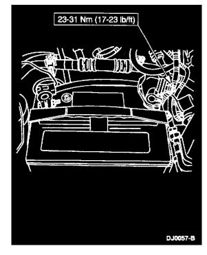
2. Unwrap the secondary positive cable and reconnect it to the primary battery terminal.
