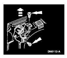
4. Remove the bolts, and remove the upper latch and cable.
