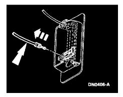
3. Disengage the cable from the door handle.
