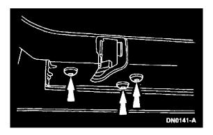
4. Remove the bolts, and remove the lower latch and cable.
