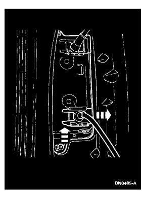
2. Disengage the lower cable keeper by pushing the bottom keeper end up and sliding the keeper toward the outside of the door.
