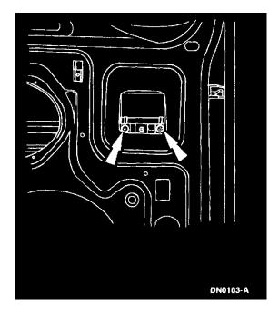
2. Remove the inside door handle nuts, and remove the inside door handle.
