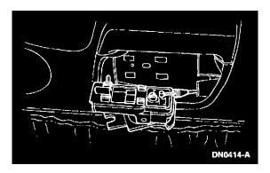
3. Disconnect the cable, and remove the latch remote control.
