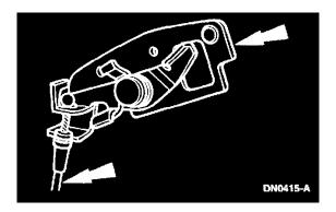
4. Disconnect the door latch cable, and remove the latch remote control.
