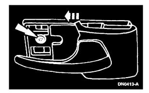
2. Remove the screw, and slide the latch remote control forward to disengage the retaining tabs from the door.
