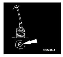
4. Drill out the power door lock actuator rivet, if so equipped.
