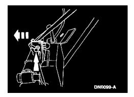
6. Front and side hinged doors: disconnect the outside door handle-to-latch rod at the door latch.
