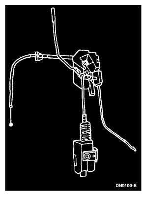
11. Front door: remove the door latch, latch remote control cable, lock cylinder rod, push-button rod and power door lock actuator, if so equipped, as an assembly.
