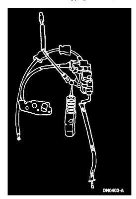
12. Side hinged and rear doors: remove the door latch, door latch remote control and cable(s), lock cylinder rod, push-button rod and power door lock actuator, if so equipped, as an assembly.
