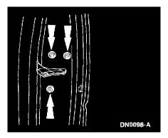
9. Remove the door latch retaining bolts.
