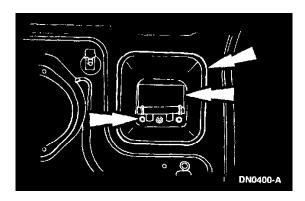
3. Side hinged or rear door: remove the retaining nuts, inside handle and bezel.
