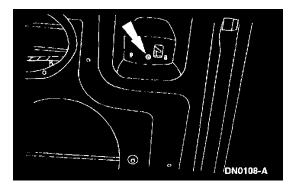
10. Side hinged and rear doors: remove the door latch remote control screw.
