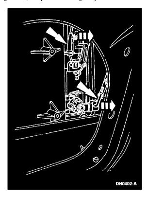
8. Rear door: disconnect the handle-to-latch cable at the door handle and the lock cylinder rod at the lock cylinder.
