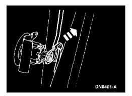
5. Front and side hinged doors: disconnect the lock cylinder rod from the lock cylinder lever.
