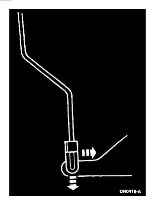
2. Disengage the retaining clip from the rod, and pull the rod away from the lever.
